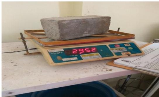
Gambar 5. Pengujian Berat Beton Kering.
